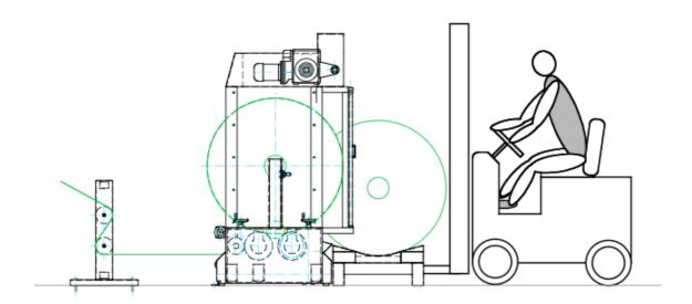
The roll is then verticalized with the Stand-up Lifter, as shown in the photo so that it can be stored on the standard pallet.
