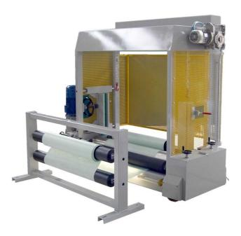
It should be borne in mind that the wrapping system makes it possible to roll up in a single direction, i.e. with the upper surface of the membrane being produced outside of the roll, for example, with the slate that can be seen when the roll is finished.
