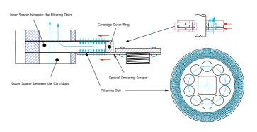
MA typed are used after the pump, installed as close as possible to the using point. The size 0,2 millimetre is especially used to filter compound which contains recovery membrane.
